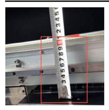
3. About guide rail: Our machine adopts Japanese THK 20mm low noise guide rail with dual sliders, more durable and reliable for high precision print. some cheap machines use Hiwin guide to reduce cost, but THK guide is much better than Hiwin guide rail.
