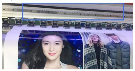
11. Our machine adopts Anti-collision performance, When the sensor installed on the both sides of the carriage detect that the position of the print head is lower than the thick medium, the carriage will initiate an immediate stop to protect the print head. Other cheap machines don't have this function.
